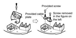
When mounting the coaxial cable in parallel with the ceiling mount, remount the provided Cable plate as shown in the figure.
